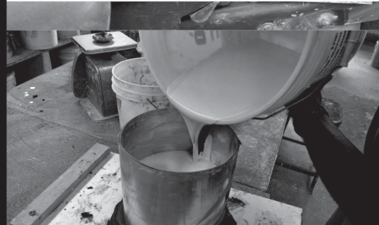
Pouring slip into a cast made from the 3D print.
