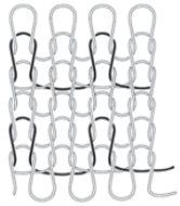
Stitches and materials to knit the textile electronic components of the radio transmitter.
