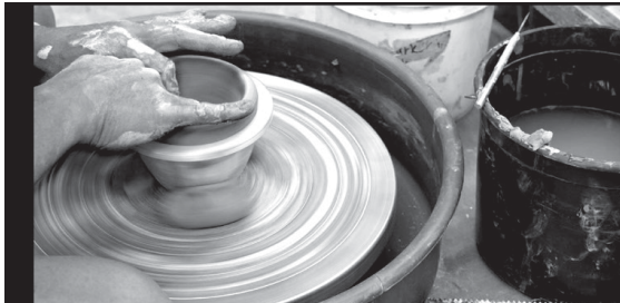
Augmenting a 3D printed form with wheel throwing.
