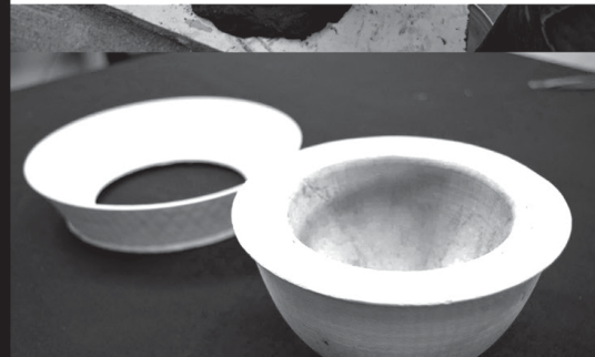
2-walled insulated ceramic bowl and 3D printed lid
